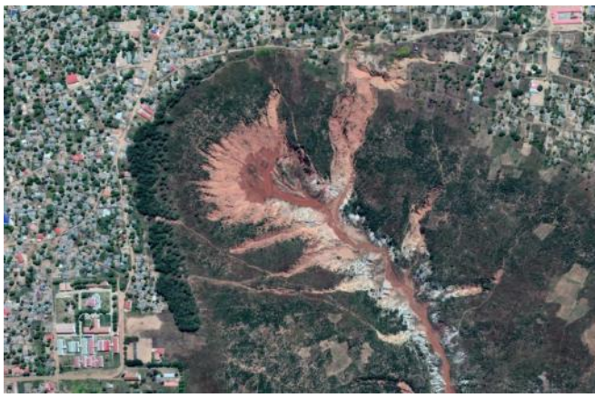
Figure 8: Around Luena soil erosion has been severe on steep slopes originally formed by slumping (see page 32). These images show the expansion of erosion in one such slump between 2003 and 2018. Note the growing density of houses around the slump. The photographs span an area of 1.6 kilometres from west to east. Source: images from Google Earth.
