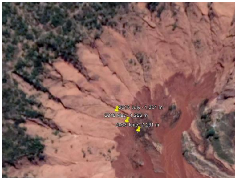
Figure 19. Slump and erosion gully at Luena (19.93 East, 11.78 South). The image was taken in May 2018, showing upper levels of ground water saturation in 2018, 2013 and 2003. The top of the saturated zone is about 60 metres below the surrounding plateau.
